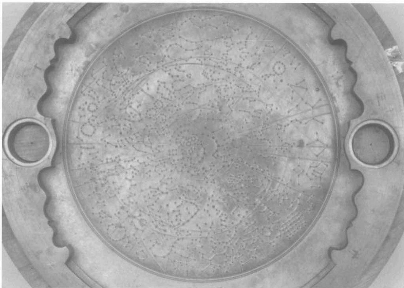
FIG. 14.5. FUKUSHIMA KUNITAKA'S BUNDO NO KIKU , 1683. This pan-shaped bronze instrument features a celestial map based on the Ch'önsang yölch'a punyajido engraved in its concave center. On the edge are two small depressions for magnetic compasses. The original was made in 1668 on the orders of the military engineer Hōjō Ujinaga. According to
